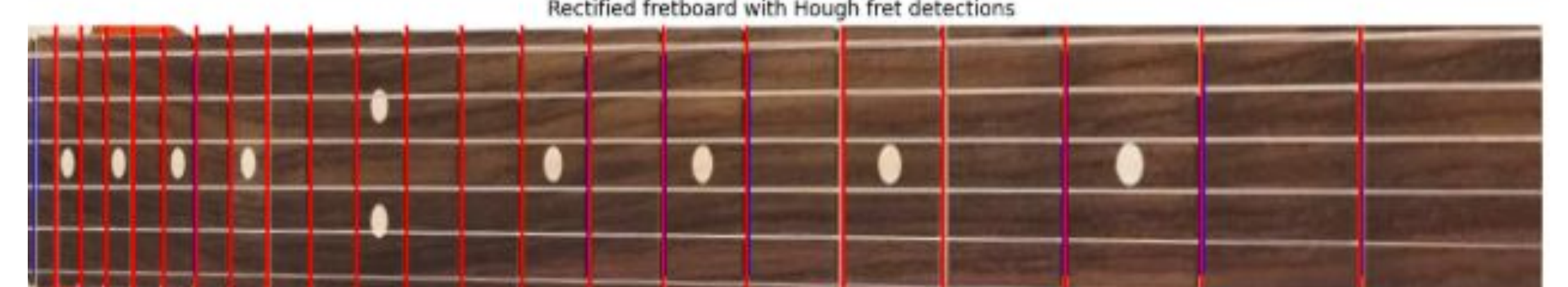
Rectified fretboard with Hough fret detections
